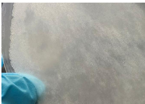
Figure 1: Picture of solid polymer electrolyte membrane based on PEO with LC as additive.
